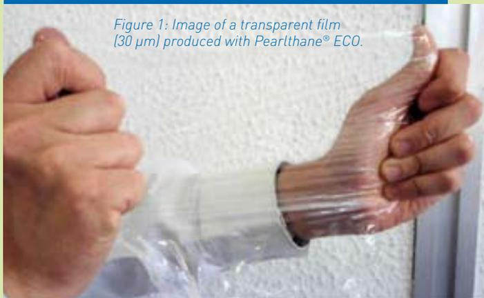
Figure 1: Image of a transparent film (30 µm) produced with Pearlthane® ECO.
